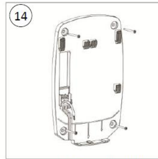
14 Screw the Plug-in base to the wall(x4)
