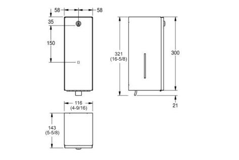
Franke Commercial 'RODAN' #RODX618 Liquid Soap Dispenser, 16-5/8" H x 4-9/16" W x 5-5/8" D (321mm x 116mm x 143mm), wall mounted, manufactured from 22 gauge (0.8mm), grade 18-10 type 304 stainless steel with satin surface finish, includes 27 oz. (800 ml) container suitable for liquid and lotion soaps, standard Franke keyed cylinder lock and mounting hardware. Provide adequate backing in wall for support and comply to local codes for barrier-free requirements.
