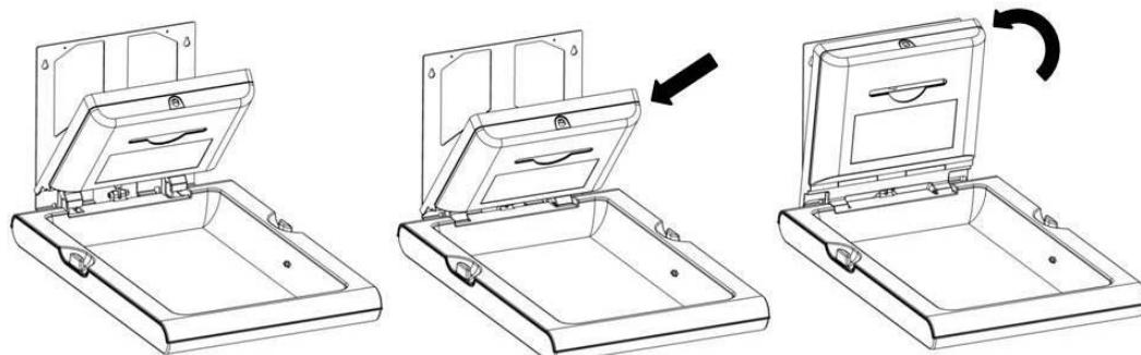
Open the liner dispenser with the special key provided. The four holes for mounting the liner dispenser on the holding structure of the changing station will be visible.
