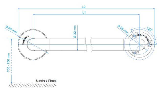
It is not recommended to install the Mediepoxy line bars in places where the bars will be in direct contact with water, in damp and/or chlorinated environments.
